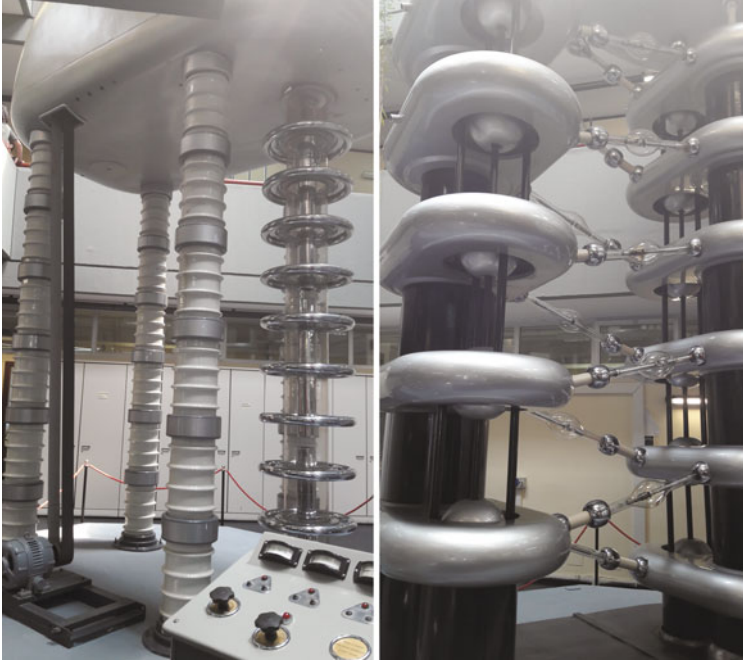
Fig. 3.6 Examples of a Van de Graaf (left) and Cockcroft-Walton (right) accelerator hosted at the LNF site
